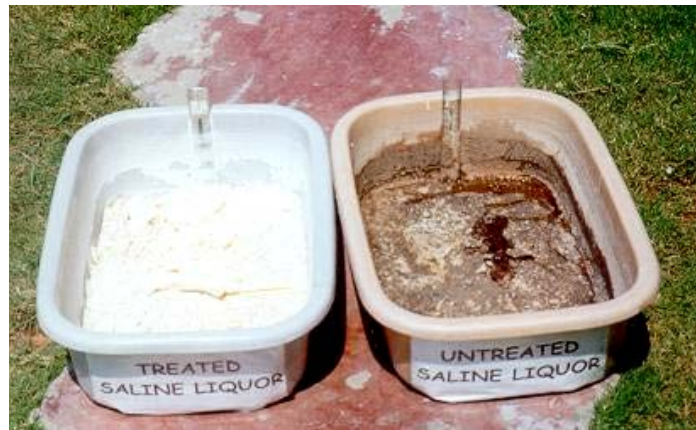
Fig. 15: Appearance of salt obtained from evaporation of treated and untreated saline effluent
