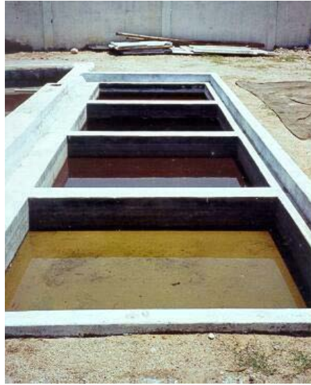
Fig. 16: Experimental solar evaporation pans
