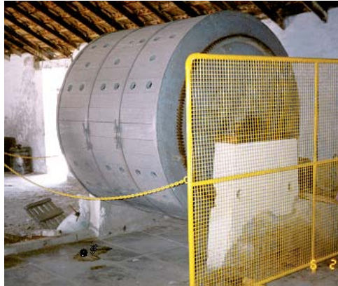
Photo 1: Mechanical desalting drum
