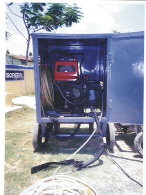
Picture 10 – Mobile air supply unit
