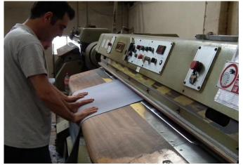
The butt part is presented grain down using a feed roller (or table).
